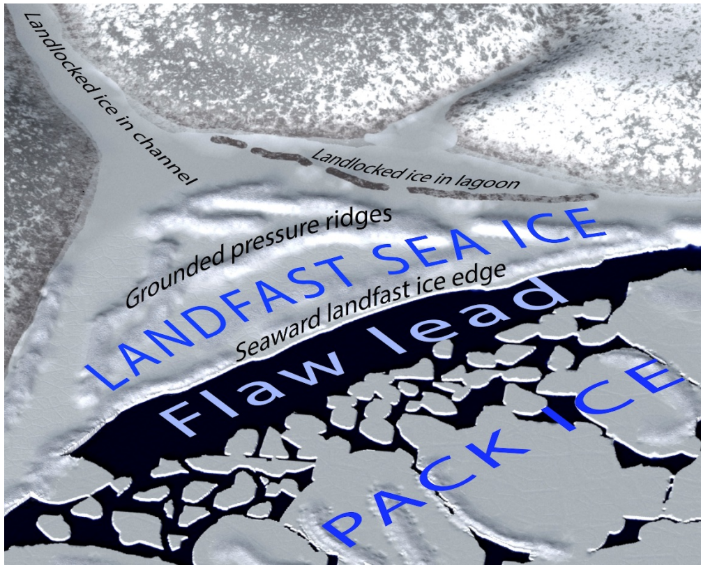
Fig. 1. Landfast ice is distinguished from the drifting pack ice by its attachment to the land. A flaw lead of open water is sometimes present at the seaward edge of the landfast ice. When the pack ice pushes against the landfast ice edge, ice deformation often occurs and creates ridges within and along the boundary of the landfast ice.
